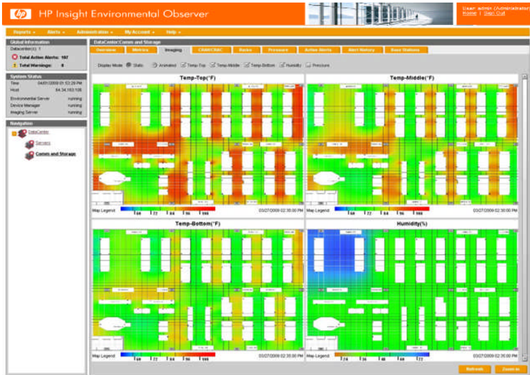
Figure 13. Visualization of the data center environment using HP Insight Environmental Observer
