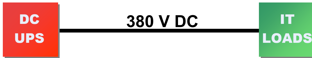
Figure 1d – Hypothetical approach for distributing 380 V DC
