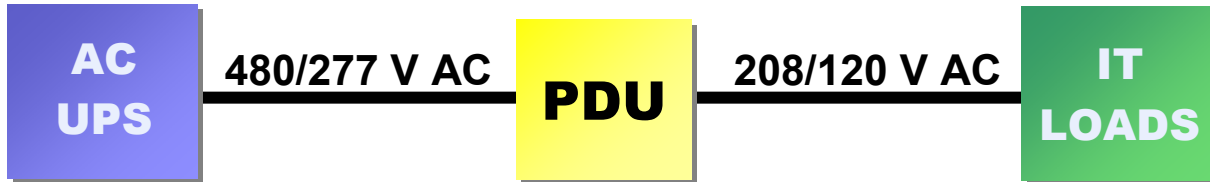
Figure 1a – Common AC distribution in North America
