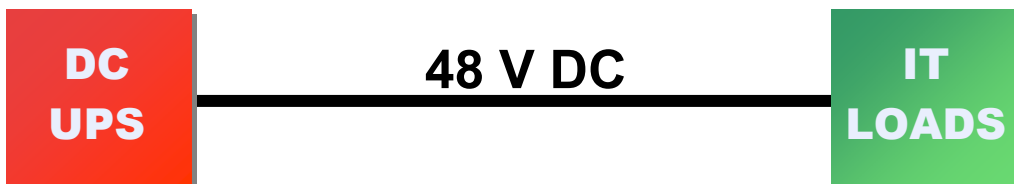
Figure 1c – Typical telecom DC distribution
