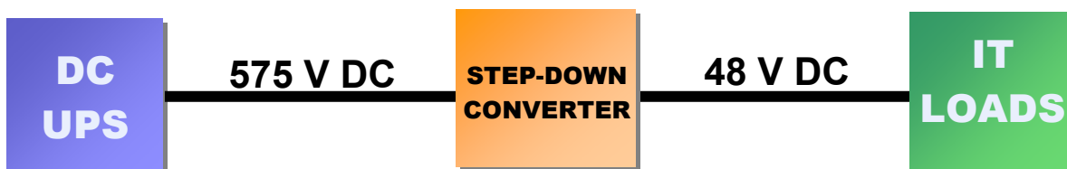
Figure 1e – Hypothetical hybrid 575 V DC system
