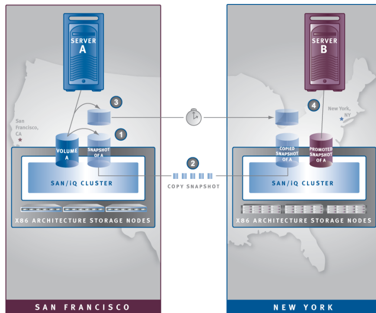
Figure 4: Remote Copy uses space-efficient, thin-provisioned snapshots to create consistent, point-in-time copies for centralized backup and disaster recovery.
